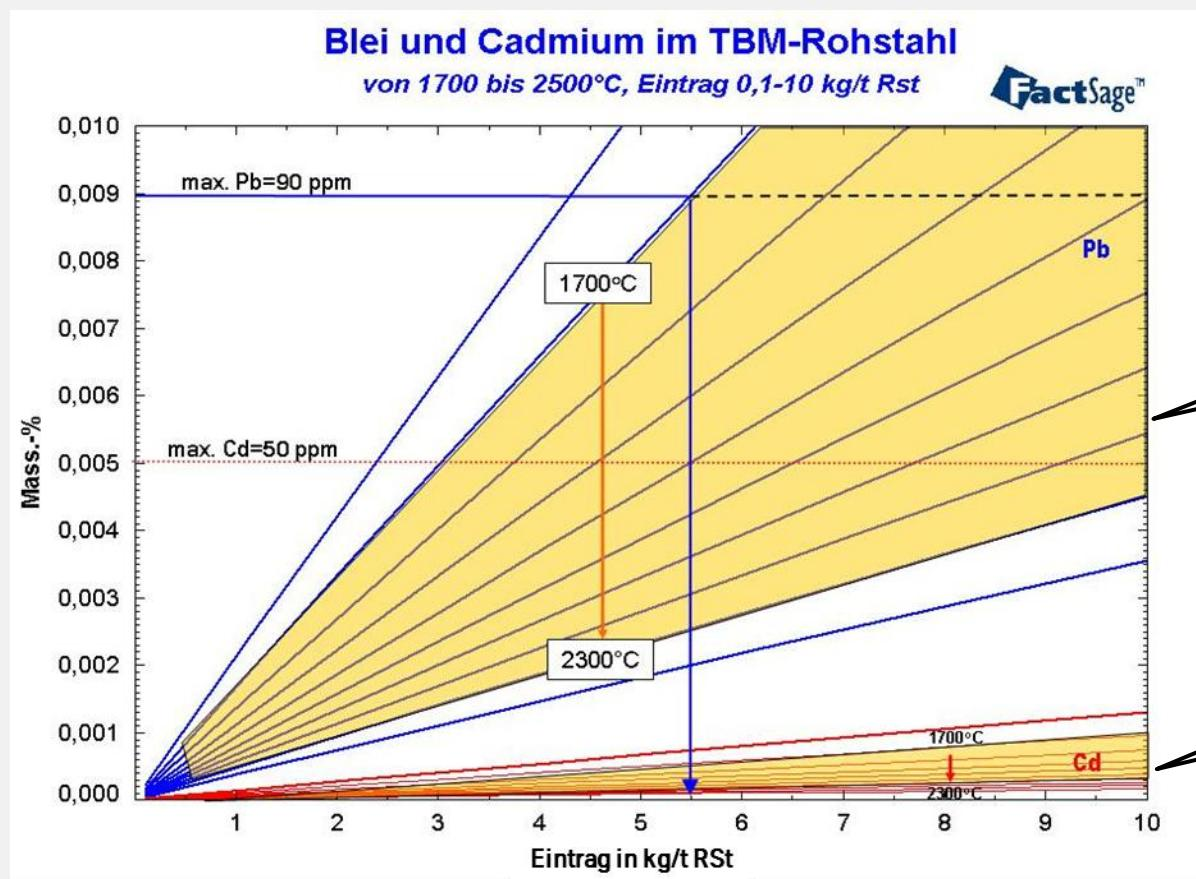
Maximum solubility of 90 ppm Pb at 1700°C can not be achieved by BOF process. An input of ca. 5,5 kg/t heavy metal is not realistic.
