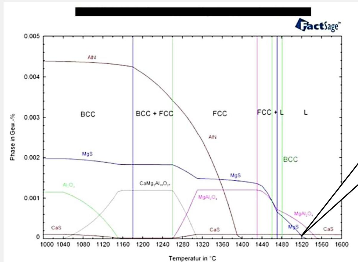
MgS is thermodynamically stable below 1520°C. Critical configurations of MgS can be avoided by reducing the Mg-content.
