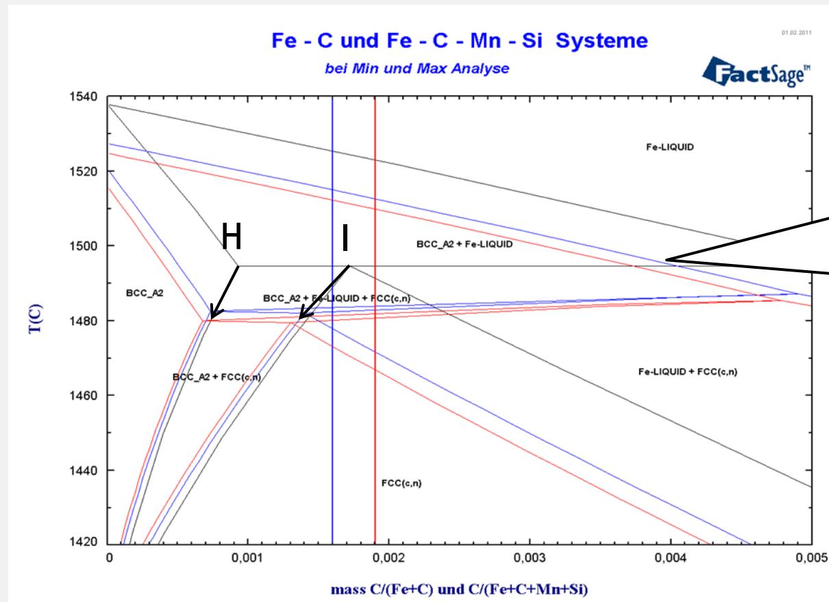
Prediction of the peritectic behaviour and prevention of the critical concentrations by adjusting the chemical composition
