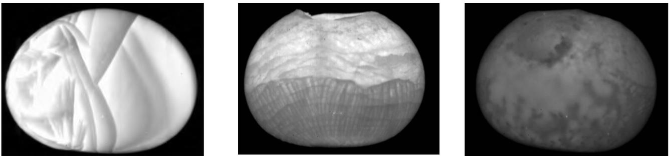
**Fig. 5:** Three different microstructures resulting from the crystallization of an undercooled YAG composition
