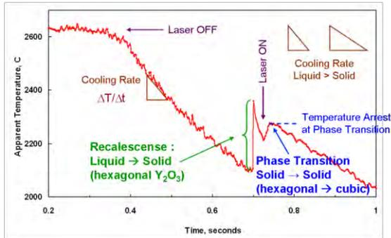
**Fig. 3:** Undercooling, Crystallization and Phase Transition of  $Y_2O_3$  (above)
