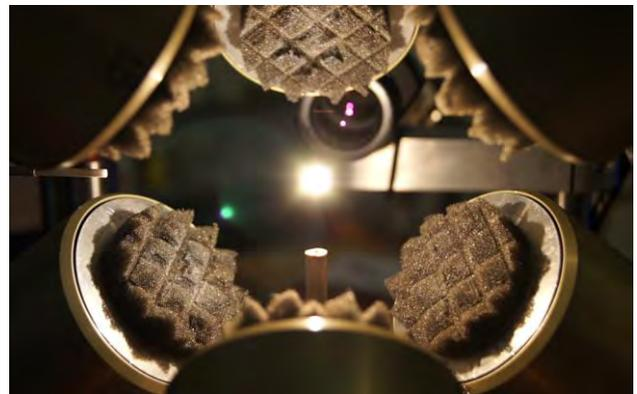
**Fig. 2:** Levitated liquid Al<sub>2</sub>O<sub>3</sub> at 2400°C
