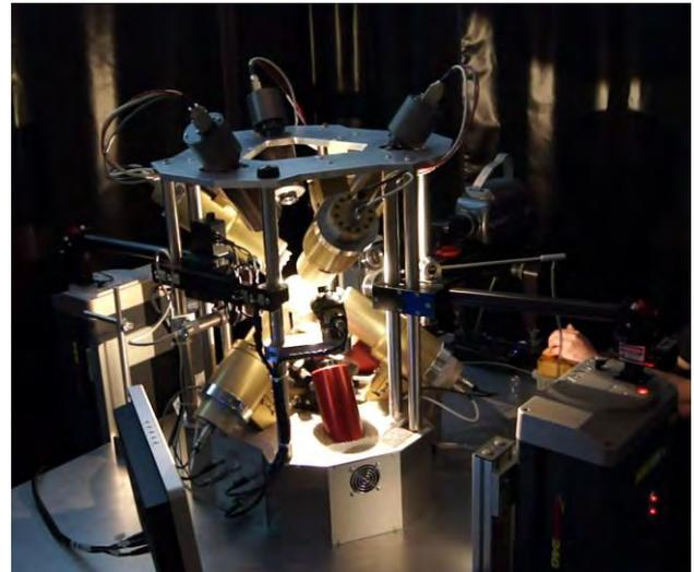
**Fig. 1:** The Aerodynamic-Acoustic Levitator
