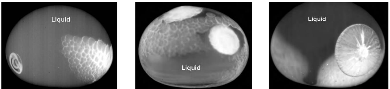
**Fig. 6:** Undercooling and Crystallization of 50:50 wt-%  $Al_2O_3:ZrO_2$  and of mullite ( $Al_6Si_2O_{13}$  / outer right)
