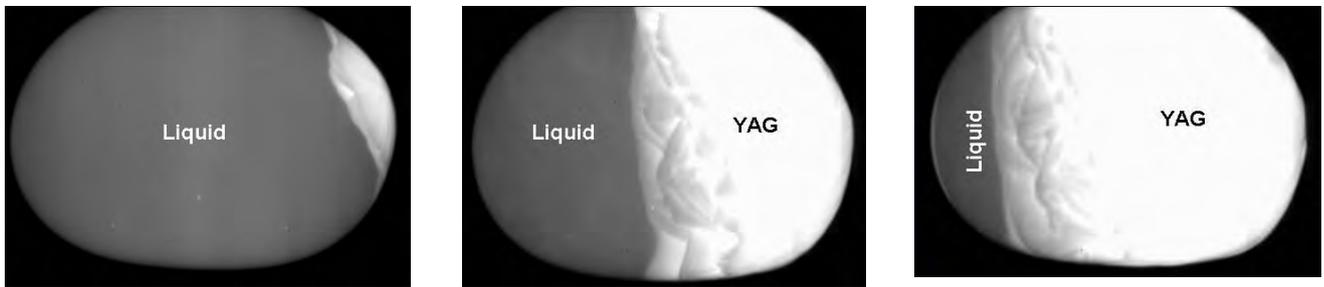
**Fig. 4:** Crystallization sequence of  $Y_3Al_5O_{12}$  (YAG) for a time period of 0.138 seconds
